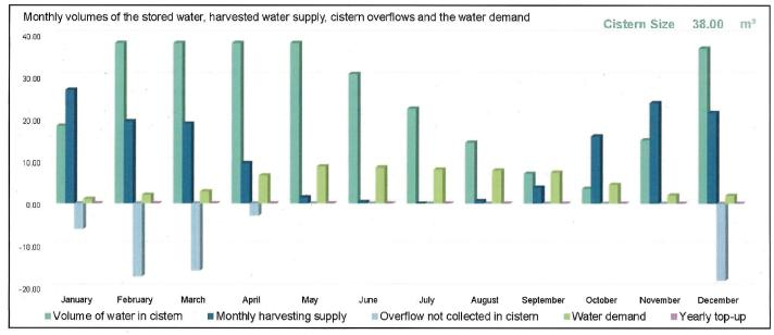
This graph represents the complexity of the rainwater harvesting calculations aimed at designing the optimal size for a water collection cistern. It incorporates the monthly runoff supplies from rain, water demands for the selected water needs, collected water level at the beginning of each month and the potential water collection surplus or additional water top-ups, if needed.
