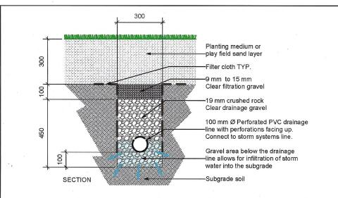
This drainage section was specially designed for maximising water infiltration into the sandy subgrades. The natural grass sports complex equipped with this simple drainage solution does not require a large and costly system to remove runoff from the 12 playing fields, and more importantly allows for maintaining pre-construction water quality and levels at the natural wetland adjacent to the site.
