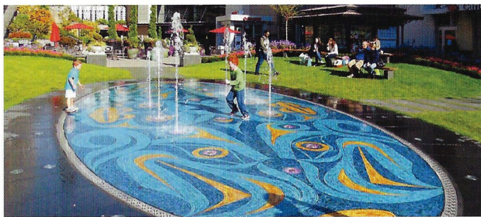
This pre-programmed dancing water element incorporates mosaic as public art and invites the public to engage with it. Each jet has an integrated LED light that is synchronised with the splashing water patterns.
